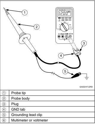
Figure 1. 80K-15 Electronic Air Cleaner Probe
